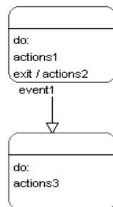
FIGURE 16. A state diagram with an exit action
